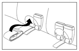
Fold the safety belt buckles and center safety belt (if equipped) into the pocket of the rear seatback.
